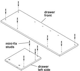
**4** ■ Use the flat-blade screwdriver and screw the mini-fix studs into the small (3/16" dia.) holes on the drawer left side, right side and drawer front.
