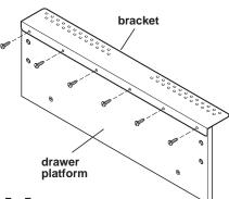
Assemble bracket to drawer platform using 6, #8 x 5/8" Phillipshead screws.
