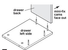
Pick up the drawer back and turn it so the mini-fix cams face out. Slide the edge holes over the rear two mini-fix studs on the drawer left side.
