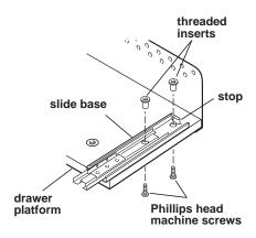
Place slide base over platform holes. Push threaded inserts through slide base into the platform holes. Tap with rubber or plastic mallet if needed. From the back of platform, thread Phillips-head machine screws into inserts and tighten securely. The stop must be at the back of the drawer platform. Repeat with other slide base.
