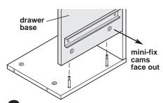
● Pick up the drawer base and turn it so the mini-fix cams face out. Slide the edge holes over the two remaining mini-fix studs.
