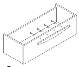
**9** ■ Insert the handle studs into the drawer front holes. Attach with pan head screws and flat washers from the back of drawer front.
