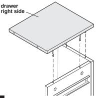
Pick up drawer right side piece and insert mini-fix studs into edge holes of the drawer base and drawer back.
