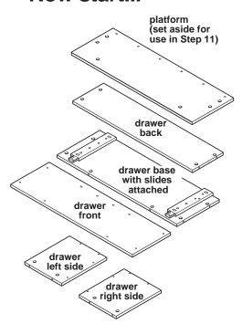
Place a protective covering on a flat surface. Remove parts bag from carton. Lay all drawer pieces except drawer platform on the covering with the holes facing up. Set drawer platform aside. It will be used later.
