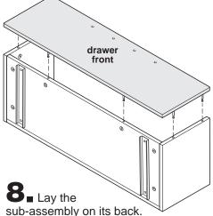
Pick up the drawer front and insert the mini-fix studs into the edge holes of the drawer sides and drawer bottom.
